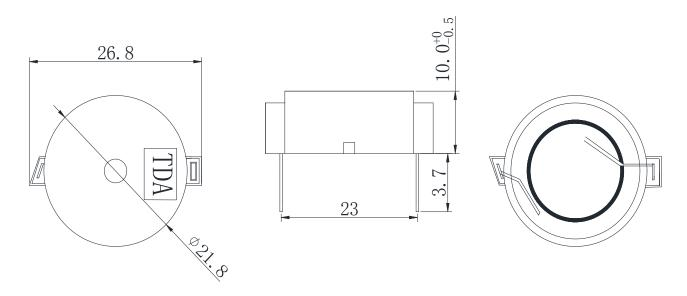
Unit:mm Tolerance: ±0.5mm
